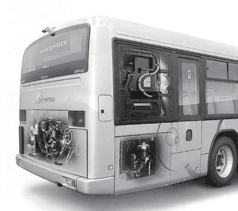
Fig. 4 Layout of Isuzu Erga Hybrid.
