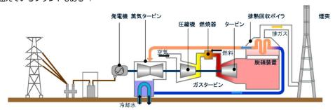
Fig 3 Schematic diagram of Combined Cycle Power Plant
