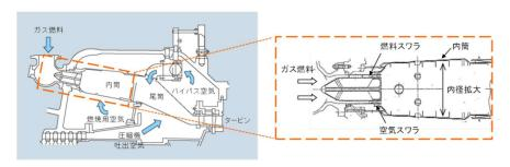
Fig 8 Diffusion-flame combustor for BFG
