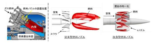
Fig 5 Improved fuel nozzle for highly-efficient gas turbine
