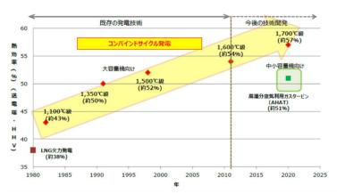
Fig 4 Improvement of Gas Turbine Combined-cycle system Thermal Efficiency
