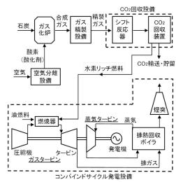
Fig 6 Schematic diagram of CCS-IGCC
