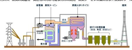
Fig 2 Schematic diagram of Steam Electric Power Plant
