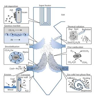
Fig. 2 Physical phenomena in a pulverized coal fired boiler
