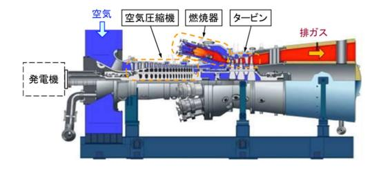
Fig 1 Schematic diagram of industrial gas turbine
