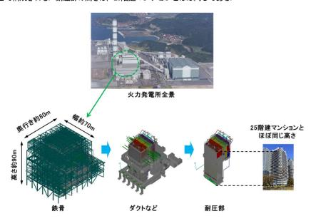
Fig. 1 Overview of a coal fired boiler for a power generating station
