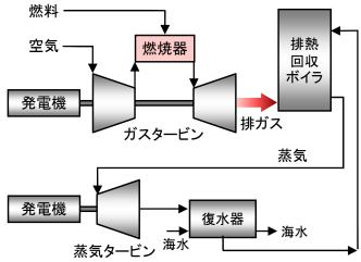
Fig 2 Schematic diagram of gas turbine combined cycle (GTCC)
