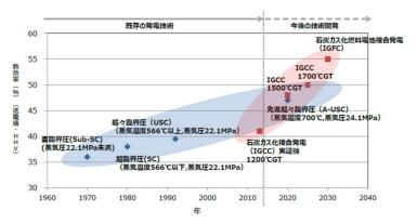
Fig 5 Improvement of Coal-fired plant thermal efficiency
