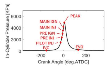
Fig. 7-1 Discretion of engine cycle
