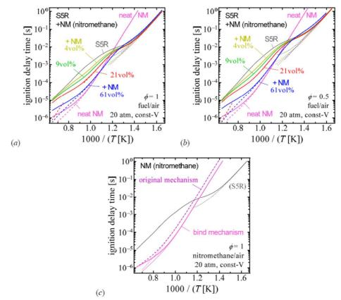
Fig. 9-2 Calculated constant-volume ignition delay times of air mixtures of nitromethane and blends with gasoline surrogate S5R. (a)  $\phi = 1.0$ , 20 atm. (b)  $\phi = 0.5$ , 20 atm. (c) comparison with original model
