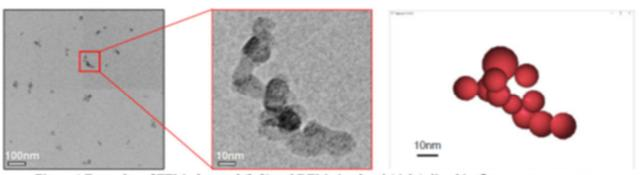
Figure 4 Examples of TEM-observed (left) and DEM-simulated (right) diesel in-flame soot aggregates
