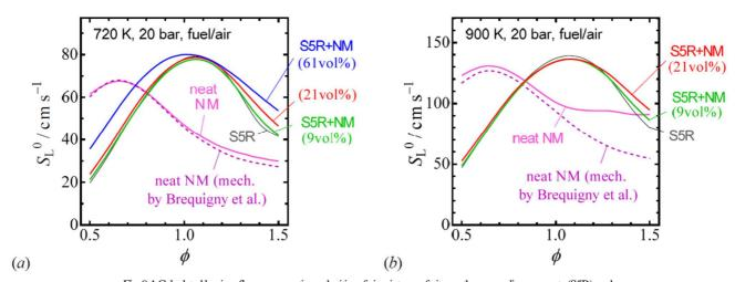
Fig. 9-1 Calculated laminar flame propagation velocities of air mixtures of nitromethane, gasoline surrogate (S5R), and nitromethane blended with S5R. (a) 720 K, 20 bar. (b) 900 K, 20 bar.
