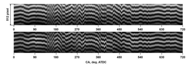
Fig 6-3 Fringe image (one cycle in continuous combustion; upper  $\lambda 1$ =515 nm, lower  $\lambda 2$ =561 nm)
