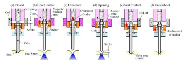
Fig.8-1 Valve behavior of injector
