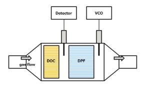
Fig. 3-5 Microwave sensor system
