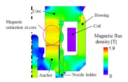
Fig.8-2 Magnetic flux density of static magnetic field
