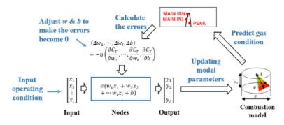
Fig. 7-2 The flow of automatic adaption
