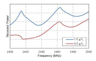
Fig. 3-6 Spectral change depending on PM accumulation
