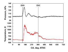
Fig 6-4 Temperature history (combustion cycle)
