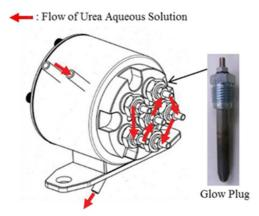
Fig. 3-2 Structure of Second Urea Reformer
