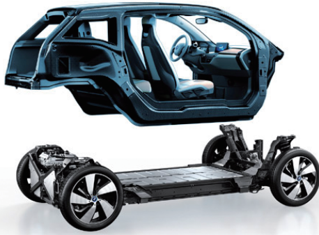
Fig. 10 BMW i3 LifeDrive chassis architecture.
