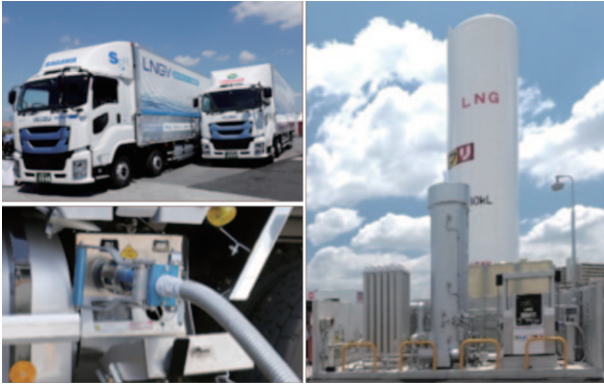
Fig. 1 LNG Trucks and L-CNG Station Built for the Project
