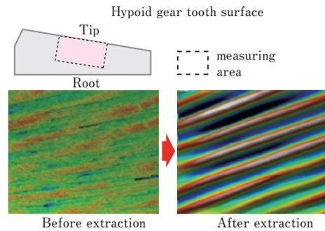
Fig. 2 Result of Extracting Tooth Surface Waviness<sup>(11)</sup>
