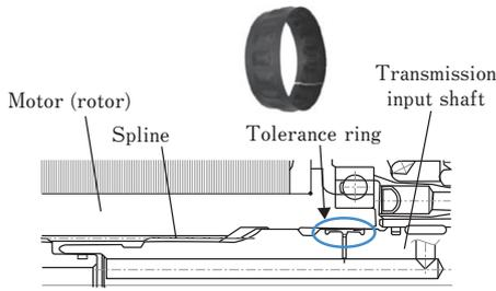
Fig. 4 Application of Tolerance Ring<sup>(14)</sup>
