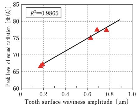
Fig. 3 Correlation between Extracted Amount of Tooth Surface Waviness and Level of Sound Radiation<sup>(11)</sup>
