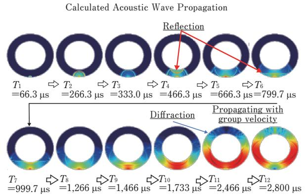
Fig. 5 Calculated Results of Sound Wave Propagation within Tire Cavity<sup>(18)</sup>
