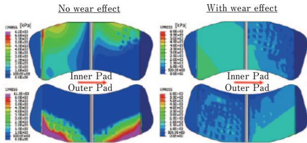
Fig. 6 Calculated Results of Surface Pressure Changes due to Lining Wear<sup>(20)</sup>
