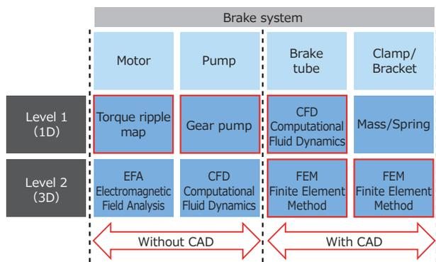
Fig. 4 Component Elements Required for Operating Noise Prediction and Modeling Method<sup>(20)</sup>
