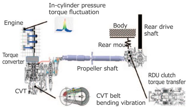
**Fig. 3** Conceptual Diagram of Prediction Model for Drive System Vibration Transmission<sup>(13)</sup>
