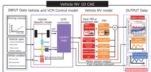
Fig. 2 1D CAE Model Integrating a Vibration Noise Model with an Engine Control Model<sup>(11)</sup>
