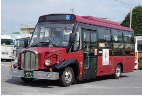
Fig. 12 Cab-Behind-Engine Electric Bus by Ono Engineering
