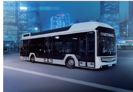
Fig. 27 Portuguese CaetanoBus H2.CityGold Equipped with the Toyota Fuel Cell System
