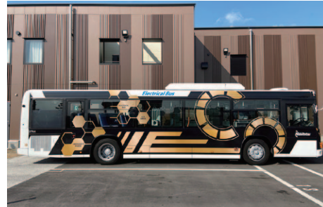
Fig. 14 Retrofit Electric Bus Converted from a Diesel Bus Starting Operation at Nishi-Nippon Railroad
