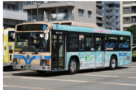
Fig. 15 Retrofit Electric Bus Converted from a Diesel Bus Starting Operation in Yokohama
