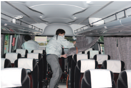
Fig. 4 Example of Applying Photocatalytic Coating to the Inside Wall
