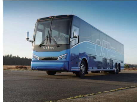
Fig. 26 Van Hool CX45E Long-Distance Electric Bus with a Range of 500 km on a Single Charge
