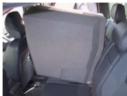
Verification that ISO 13216-3 fixtures do not interfere with the vehicle's interior components and parts (under review in WG2)
