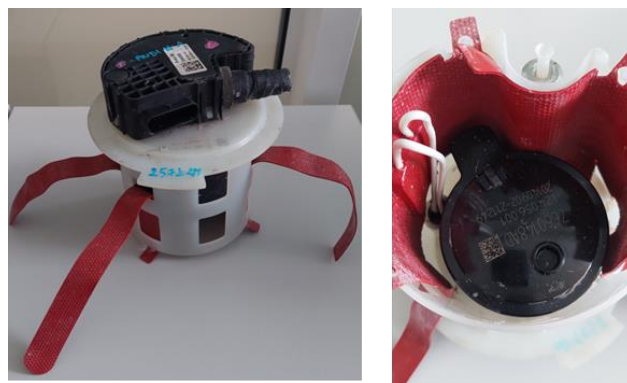
Fig.1 Gen-II ADM pump after 12 years and 257,000 km, ready for a next vehicle life
