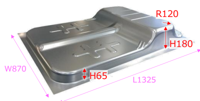
Fig.2 Prototype of the upper cover made of Zn-Al-Mg coated steel sheet
