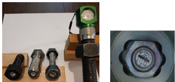
Fig. 3 Axial force indicator bolt
