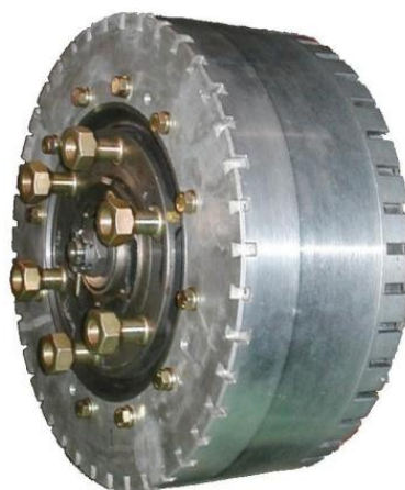
Fig.4 Outer rotor type 22.5-inch in-wheel motor.
