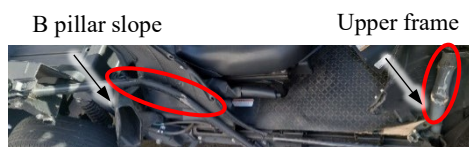
Fig.2 Vehicle deformation
