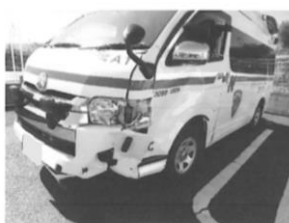
Fig. 2 Deformation of ambulance
