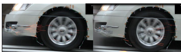
Fig.1 Flow visualization using light emitting particles
