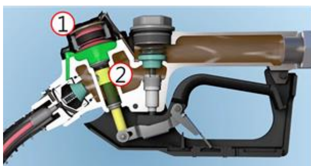
Fig.1 Dispenser Nozzle Shut Off Mechanism off by fuel
