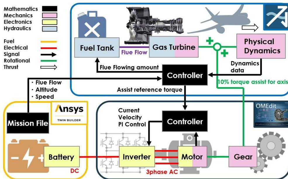
図 2.1.1-1 Hybrid aircraft's system simulation model
