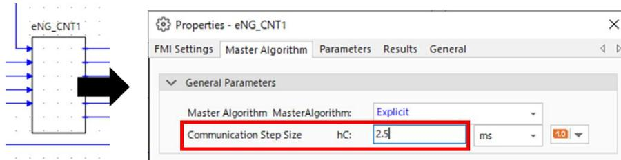
図 1.6.3-2 Properties > Master Algorithm > Communication Step Size
