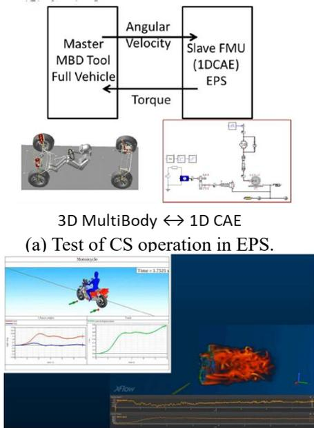
図 2.2.3-1 3D (slave) with 1D simulation.
