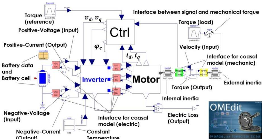
図 2.1.2-1 Electrical Drive Block Model
