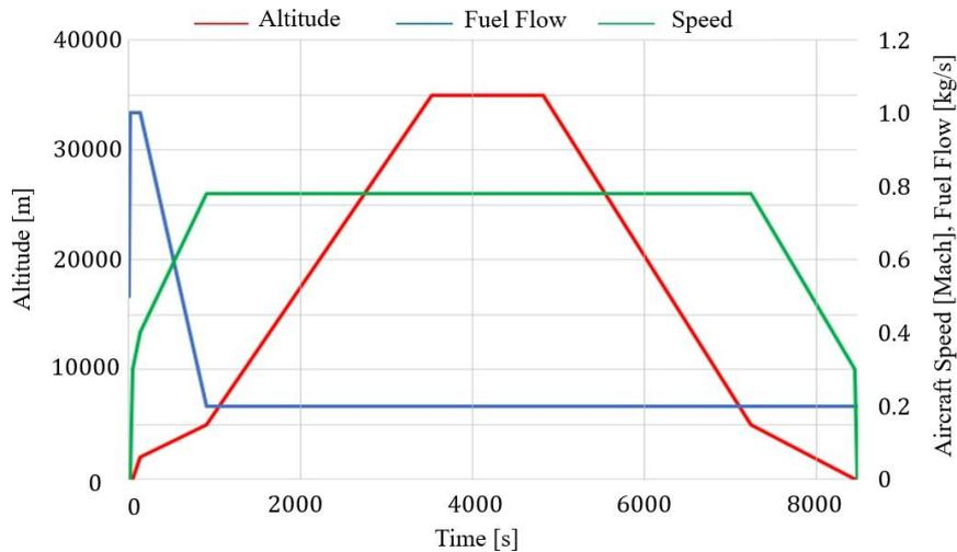
図 2.1.3-1 Flight profile (input data)
