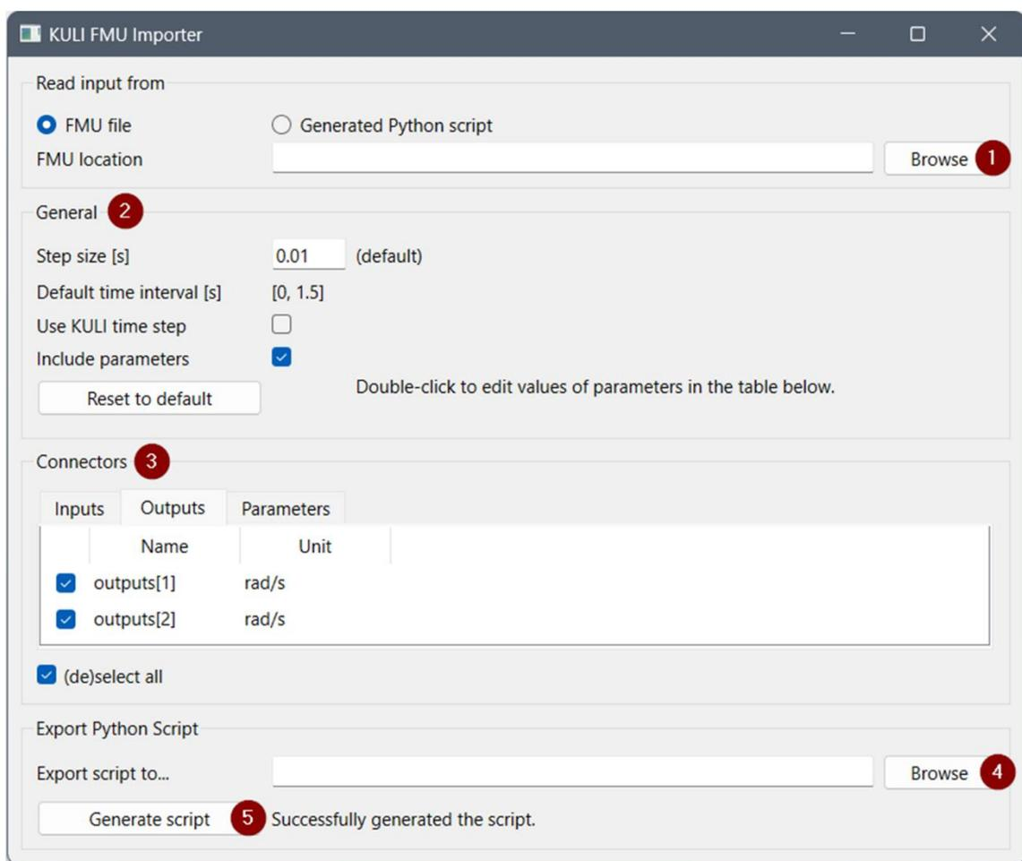
図 1.13.2-1 Start\_Script\_Generator.bat GUI
