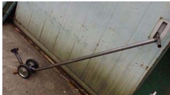
**APPENDIX J-IN-1 Special caliper for measuring laminate thickness (J2026-IN-08)**
