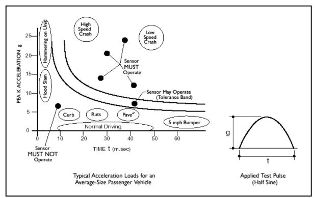
Above are the typical performance characteristics of resettable crash sensors
