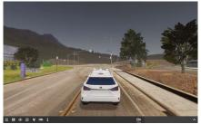
The team's vehicle must avoid a vehicle parked on the shoulder upon approaching to a target distance of 1.2 m, and go past the checkpoint ahead of the parked vehicle within the predetermined time.
