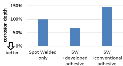
Fig.2 Corrosion depth of lap-joint of GA steel plates under Cyclic Corrosion Test
