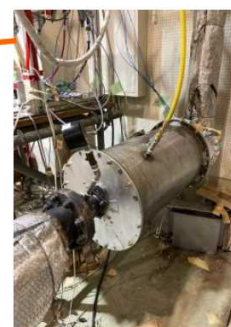
DPF with vacuum insulation device (The size of diameter and length is almost equal to normal DPF)
