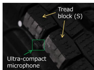
Fig.2 Measurement of sound pressure in the sub-grooves of the tread blocks using an ultra-compact microphone
