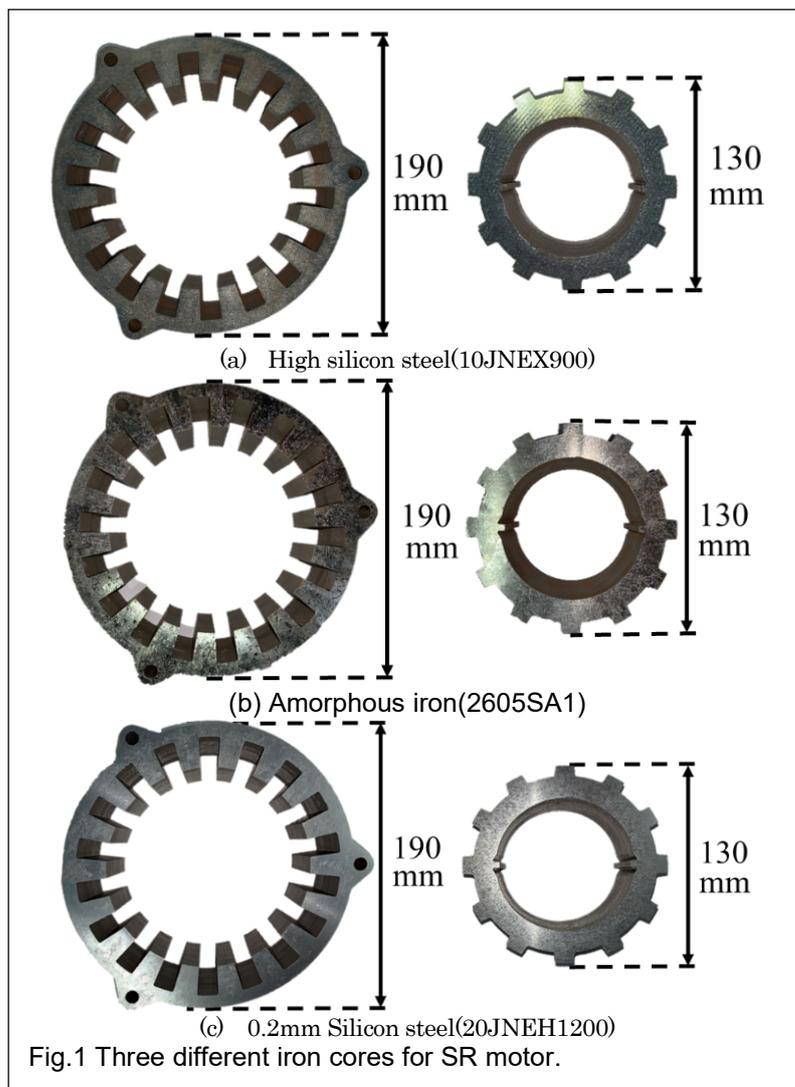
Fig.1 Three different iron cores for SR motor.
