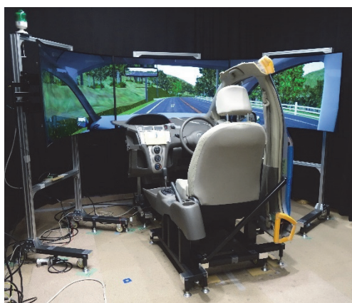
Fig.1 Real Vehicle Cockpit with Wide Visibility Driving Simulator
