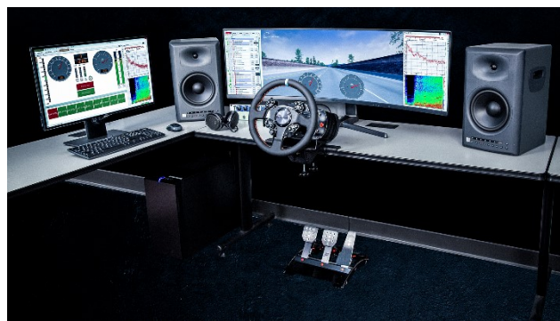
Fig. 1: driving simulator for NVH
