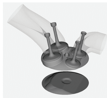
Fig.1 2Stroke Engine with Valves
