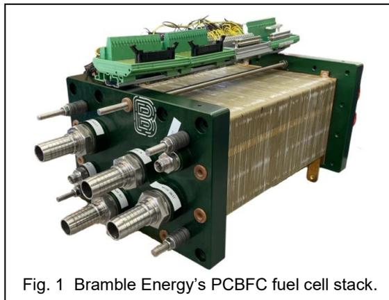
Fig. 1 Bramble Energy’s PCBFC fuel cell stack.
