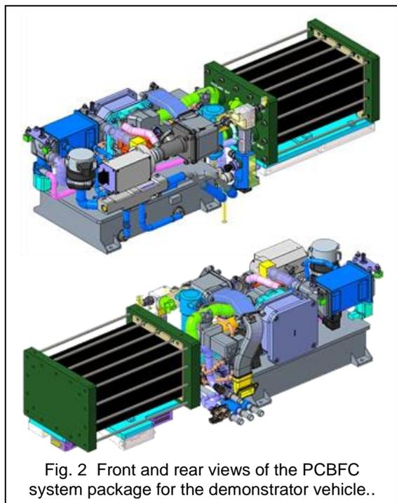
Fig. 2 Front and rear views of the PCBFC system package for the demonstrator vehicle..
