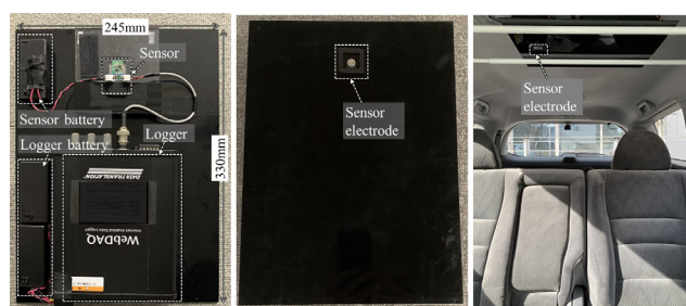
Fig.1 Sensor unit and example of placement in a vehicle cabin
