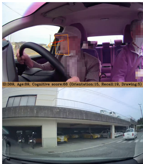
Fig.1 Driving Behavior from Video Image with Annotation of Eye Gazing Vectors and Face Position, Direction Vectors
