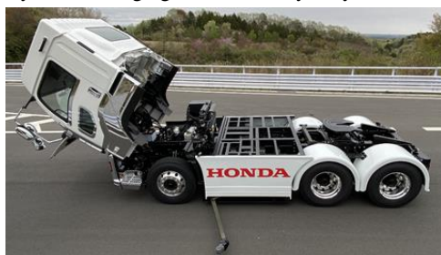
Fig.3 Dynamic Charge Power Unit Layout (6x4 Tractor)
