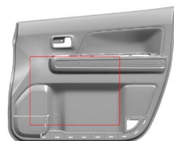
Fig.2 DIC measurement area in the door trim
