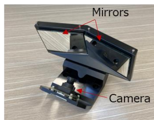
Fig. 2 Overview of prototyped monocular stereo camera
